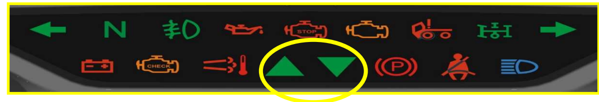
Gear Shift Advisor in Instrument Cluster
